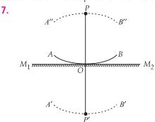
In figure, P is a point object placed at a distance r from a plane mirror  $M_1M_2$ . With P as centre and PO = r as radius, draw a spherical arc; AB. This is the spherical wavefront from the object, incident on  $M_1M_2$ .
