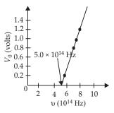
$V_0$  versus plot shows that the first four points lie nearly on a straight line which intercepts the x-axis at threshold frequency,  $\upsilon_0 = 5.0 \times 10^{14}$  Hz. The fifth point  $\upsilon$  (= 4.3  $\times$  10<sup>14</sup> Hz) corresponds to  $\upsilon < \upsilon_0$ , so there is no photoelectric emission and no stopping voltage is required to stop the current.
