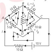
Loop 1  $\Sigma E = \Sigma I R$  $10I_1 + 5I_g - 5I_2 = 0$  or  $2I_1 + I_g - I_2 = 0$ ...(i)  $\Sigma E = \Sigma I R$  $5I_g + 10[I_2 + I_g] - 5[I_1 - I_g] = 0$  $10I_2 + 20I_g - 5I_1 = 0 \quad \text{or} \quad 2I_2 + 4I_g - I_1 = 0$ ...(ii)
