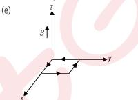
Dipole moment is along + z direction.  $\vec{\tau} = \vec{M} \times \vec{B} = 1.8 \times 10^{-2} \hat{k} \times \hat{k} = 0$ Potential energy  $U = -\vec{M}.\vec{B}$
