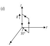
Dipole moment is at an angle 150° with the +x direction.
