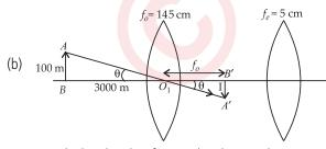
We can calculate height of image by objective lens
