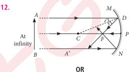
A ray passing through centre of curvature of a concave mirror gets reflected along the same path because it falls along normal to the surface of mirror, and we know that any ray passing through normal reflects along the same path.
