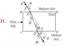
A light ray incident on a rectangular glass slab immersed in any medium emerges parallel to itself because the extent of bending of the ray of light at the opposite parallel faces *AB* (medium-glass interface) and *CD* (glass-medium interface) of the rectangular glass slab is equal and opposite.
