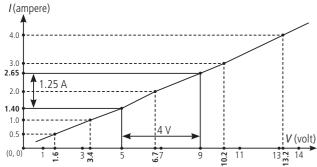
For finding R consider any two sets of values for V and I For  $V_1 = 10.2$ ,  $I_1 = 3$
