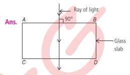
**16.** How does the lateral displacement of emergent ray depend on the width of the glass slab and angle of incidence?
